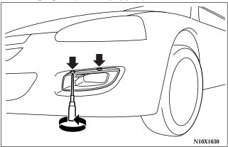
1. Insert a screwdriver as shown in the illustration and 8 remove the screws.
